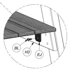
Step 2: Attach Floor Assembly to 'H3' floor braces using screws 'BL', as shown.
