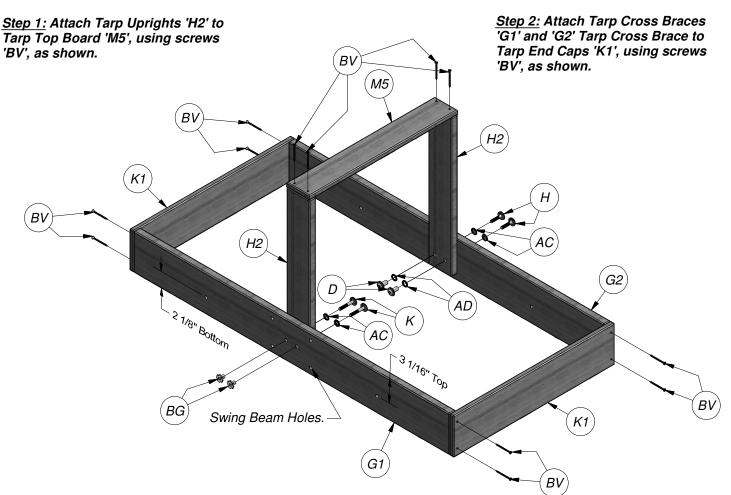
Step 3: Attach Tarp Upright 'H2' to Tarp Cross Brace 'G2', using hardware 'H', 'AC', 'AD', & 'D', as shown.
