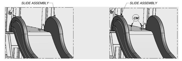
Step 1: Center the wave slide assembly in the opening opposite the swing beam assembly, as shown.
