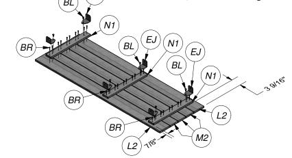
Step 1: Using 'N1' Floor Supports as a template, pre-drill & attach Floor Supports 'N1' to Floor Boards 'M2' & 'L2' approximately 3 9/16" from both edges of 'M2' boards and center the remaining 'N1' support, as shown. Attach N1 supports to 'M2' boards using screws 'BR', as shown. Finally, secure L-Brackets 'EJ' to 'N1' supports using screws 'BL', as shown.
