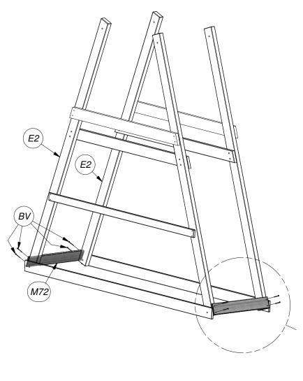
Step 1: Pre-drill & attach 'M72' Rock Wall Slat to the edges of 'E1' & 'E2' Fort Uprights using hardware 'BV', as shown.
